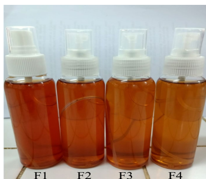
Figure 12. Four Disinfectant products with different volumes of active ingredients. F1, F2, F3, and F4 respectively contain active ingredients from a mixture of silver nanoparticles with mangosteen fruit extract of 10, 15, 20, and 25 mL.
