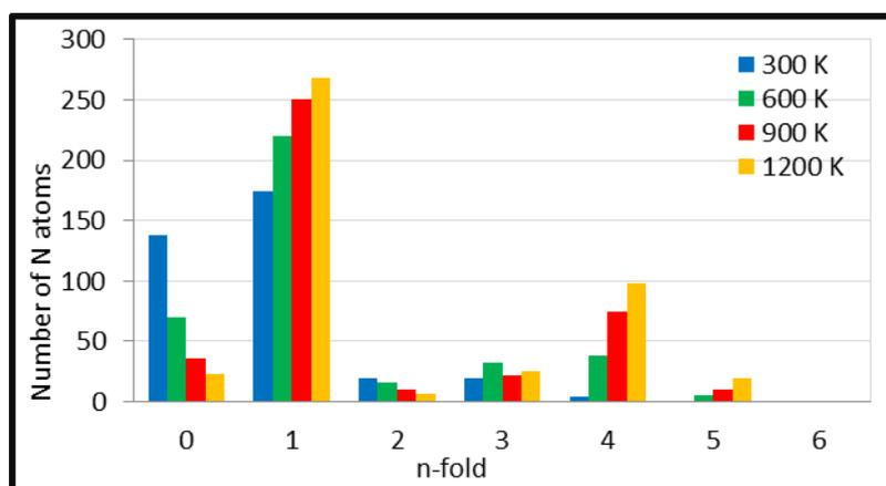
**Figure 8.** Number of n-fold coordinated N atoms after the nitrogenation process
