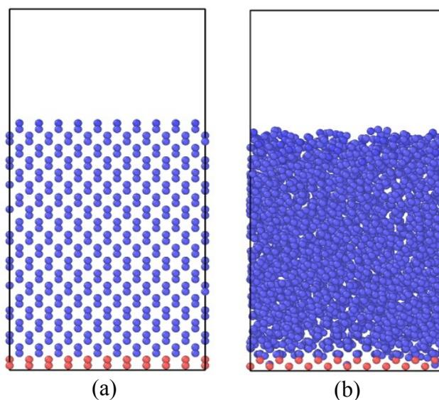
**Figure 1.** (a) Crystalline silicon structure before the amorphization process, (b) The structure of amorphous silicon after amorphization process.
