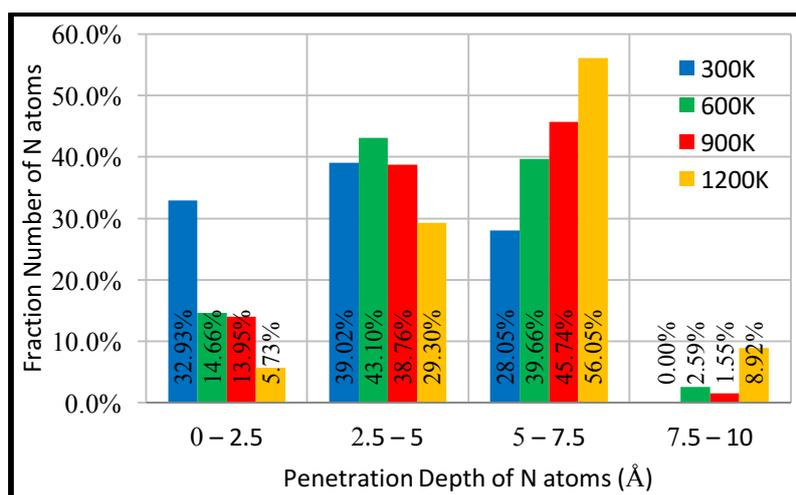
**Figure 6.** The fraction of N atoms in an nitrogenated amorphous silicon for 20 ps
