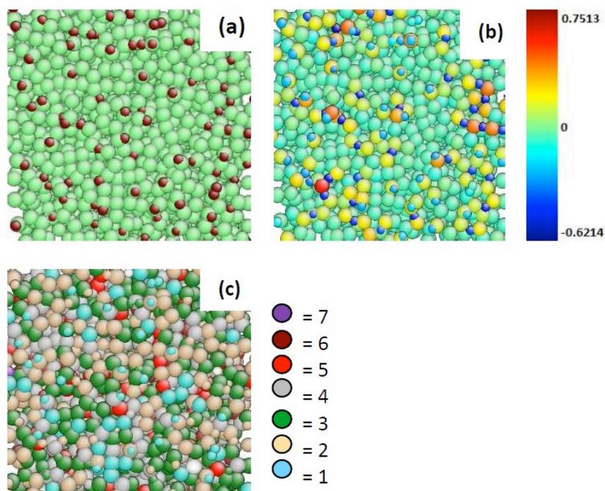
**Figure 9.** Top view of the surface of amorphous silicon nitride at 300 K: (a) atomic species (Si = green, N = dark brown), (b) atomic charge, (c) atom coordination number.
