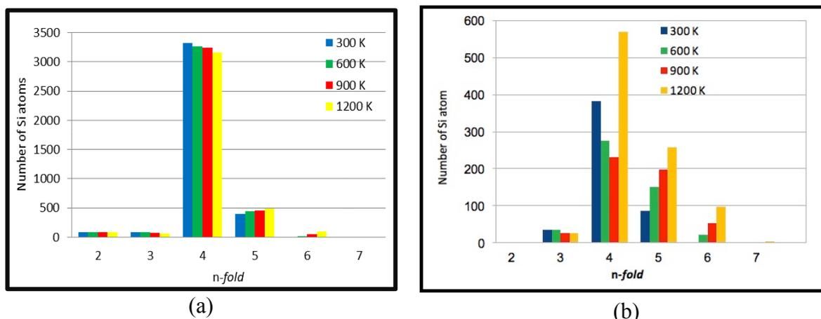
**Figure 7.** Number of n-fold coordinated Si atoms after nitrogenation in the entire silicon surface (a), and number of n-fold coordinated Si atoms after nitrogenation in the area of silicon surface which make bonding with nitrogen atoms (b).
