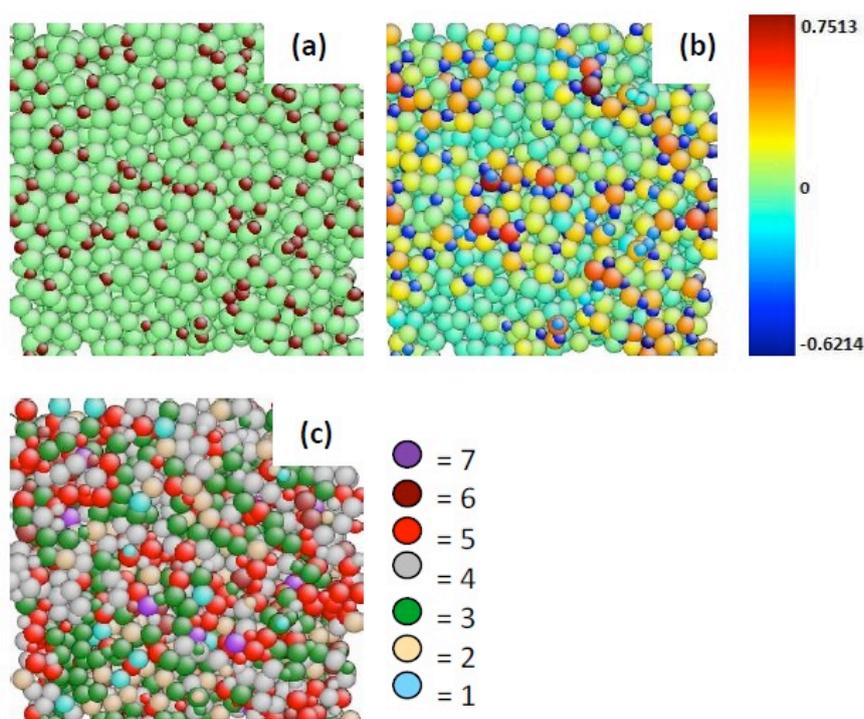
**Figure 11.** Top view of amorphous silicon nitride surface at 900 K. (a) atomic species (Si = green atoms and N dark brown atoms), (b) atomic charge, (c) atom coordination number.
