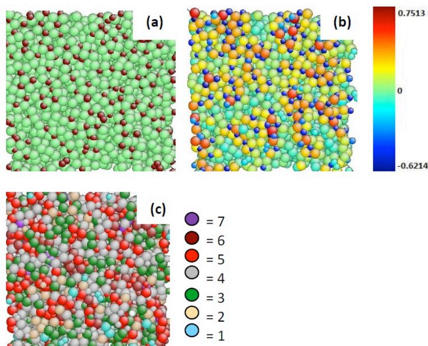
**Figure 12.** Top view of amorphous silicon nitride surface at 1200 K. (a) atomic species (Si green atoms and N dark brown atoms), (b) atomic charge, (c) atom coordination number.
