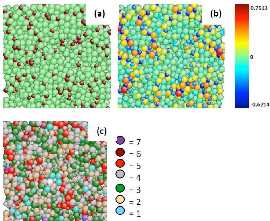
**Figure 10.** Top view of amorphous silicon nitride at 600 K surface: (a) atomic species (Si = green, N = dark brown ), (b) atomic charge, (c) atom coordination number.
