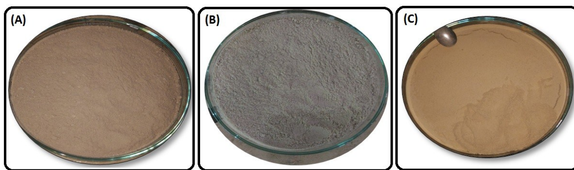
Figure 4. The powder of papyrus fiber (A), cellulose (B) and cellulose ester citrate by using 0.6M citric acid at 120 °C (C).
