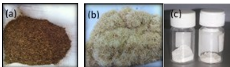
Figure 4. OPEFB (a) untreated (b) Treatment with alkali (delignification) (c) Cellulose nanocrystal
