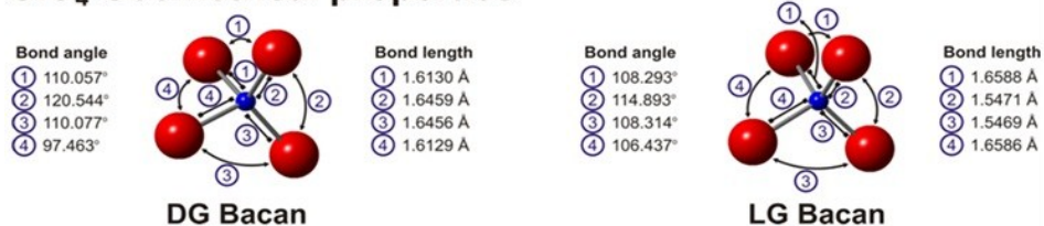
Figure 5. \text{SiO}_4 coordination bonding of \text{SiO}_2 crystal phase which represented from DG and LG Bacan.
